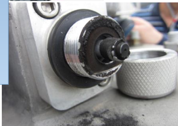
解体确认的套管末屏
